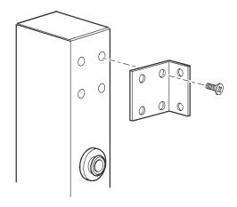
2. Attach the Rack PDU to a vertical mounting rail in the rear of the enclosure using two additional screws per bracket (not provided).
