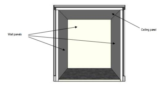
Panels will be installed on the walls and ceiling and will be composed by a sandwich of materials with fire resistance and thermal insulating to resist high temperatures and provide a watertight enclosure. The sandwich will be covered by one layer of galvanized steel sheet (0,6 mm), joined by continuous weld panel to panel.
