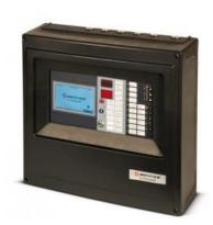
The fire panel controls the fire detection and extinguishing system. The panel can monitor two distinct areas, can trigger at least 2 levels of alarms, and incorporate a delay to evacuate the room before activating the extinguishing system. The system can also be activated by a manual switch attached to the panel.
