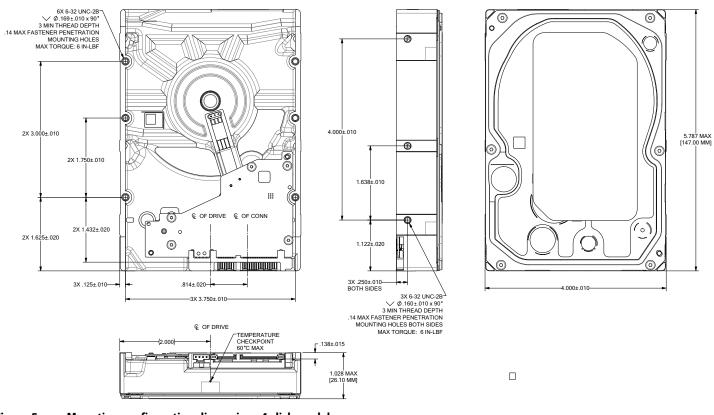
Figure 5. Mounting configuration dimensions 4-disk models
