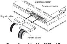
Figure 3. Attaching SATA cabling
